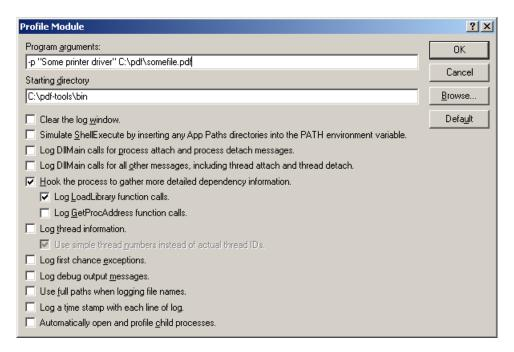
Search the log for DLLs which are loaded multiple times.
